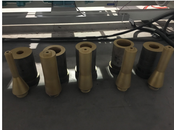
8. mould for pipe winder forming machine
