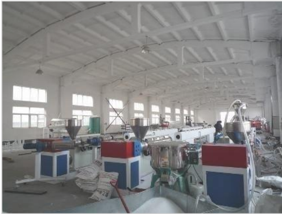
Part 2 Small pipe production line (son pipe)
