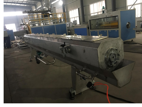
5.Spray sizing water tank
