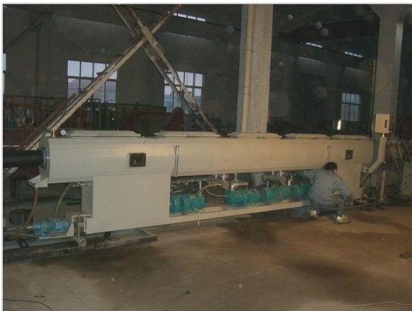
3. Vacuum calibrating spray water tank
