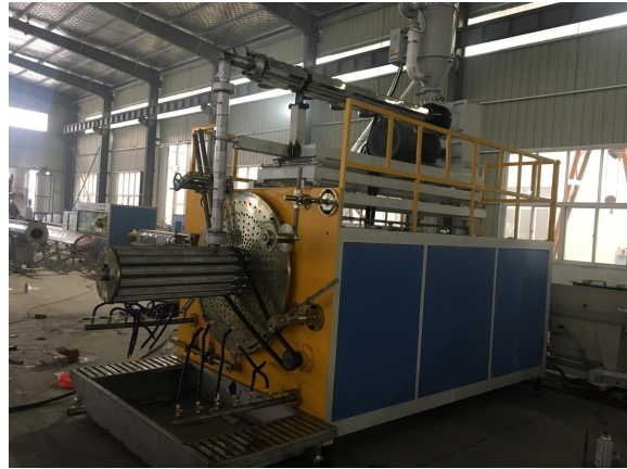
9. extruder for melting glue
