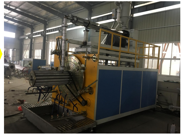
6.Winder forming machine CRGJ300—1000
