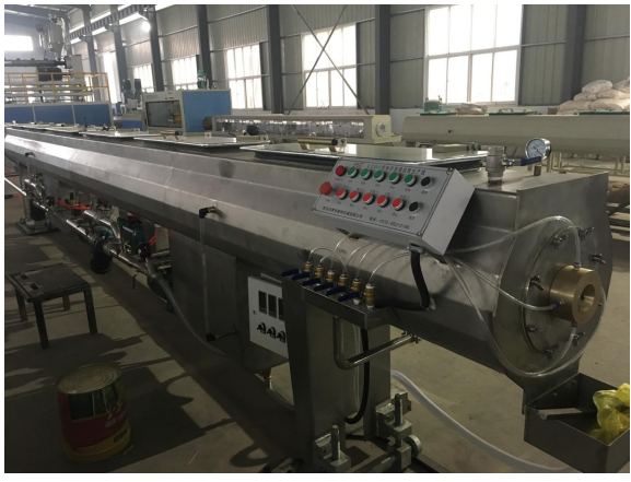
4. Vacuum sizing cooling system CRZL - 110
