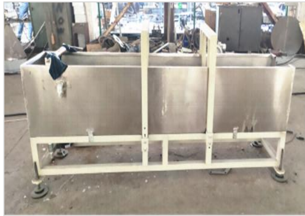
7. cooling water tank
