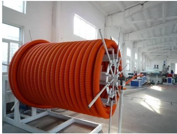
Spiral pipe production line (mother pipe)
