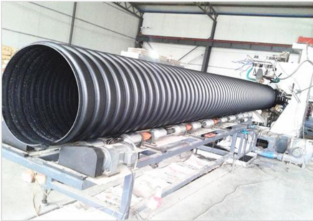
PE high speed steel strip reinforced spiral corrugated pipe
